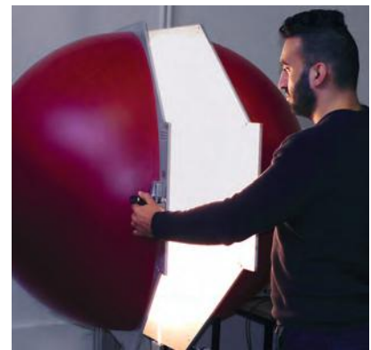
The luminous flux of the luminaires is measured in Teknoware's laboratory using an Ulbricht sphere.
